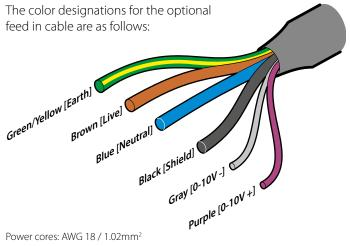
Power cores: AWG 18 / 1.02mm<sup>2</sup> Signal cores: AWG 26 / 0.13mm<sup>2</sup>
