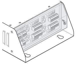
2 Disengage the upper lip of the cover from the AL Driver frame.
