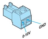
Insert the terminal block into the **ANALOG IN** socket and ensure that it fully clicks into place.
