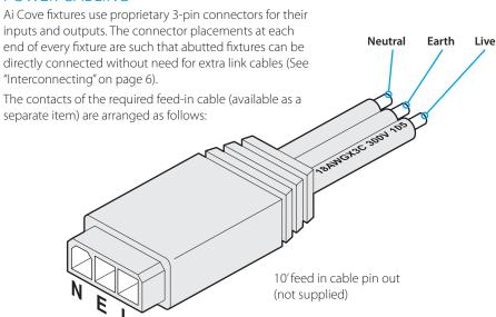
Note: Ensure that the mains power is supplied from a suitably protected source and initial connections are made within IP rated enclosures.
