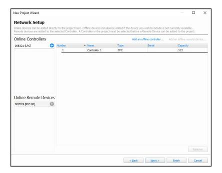
The Network Setup allows you to add any Pharos devices on the network to the project or add an offline device.
