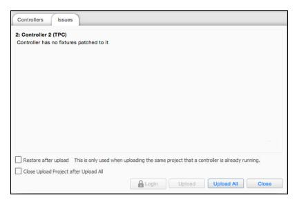
When you open the Upload dialog, there is a tab which lists potential errors with your project. Designer will check things like triggers and hardware configuration to make sure that there are no inconsistencies. If any issues are found, the Issues tab will be opened automatically and a description of each issue will be listed so that you can take corrective action, see Issues. You can proceed with the Upload ignoring the errors should you wish.
