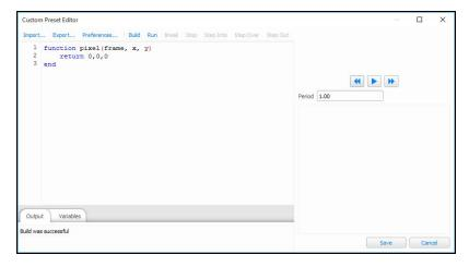
The script editor initially shows the framework of a custom preset. You can either enter the source yourself, or you can load the source from a file using Import. Designer provides sample scripts which are located in Program Files at \Pharos\Designer\resources\scripts\custom presets.
