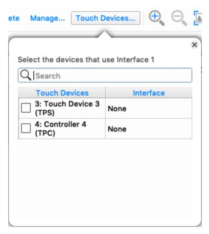
To link an Interface to a TPC/TPS, use the Touch Devices... option in the toolbar.
