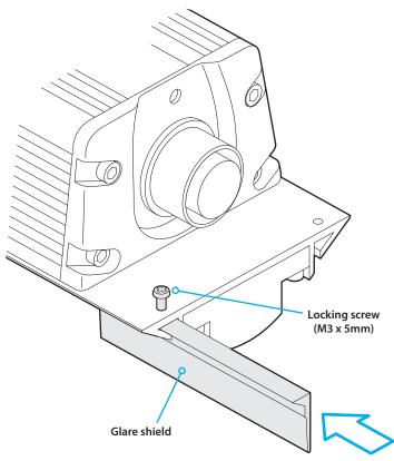
2 When the shield is fully in place, on the underside of the fixture, insert one of the supplied small locking screws at either end and tighten them to keep the shield firmly in place.
