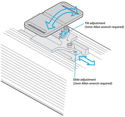
Ensure that each base is securely fixed to the mounting surface with appropriate screws/ bolts. If necessary, use a 2mm Allen wrench to loosen each mount to allow them to slide along the length of the fixture to the required position before re-tightening.
