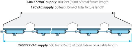
**120VAC supply**: 250 feet (76m) of total fixture **plus** cable length
