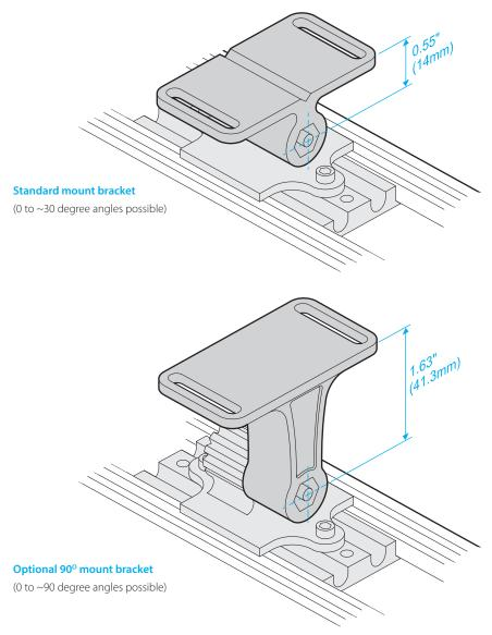
To fit the optional bracket, remove the tilt adjust bolt (5mm Allen wrench required), remove the standard bracket and replace with the new part.
