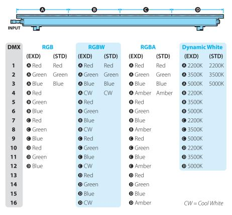
The channel allocations above are shown beginning at DMX address 1. When you configure a fixture with an alternative DMX address, that value will become the first channel in the list shown above and the other channels will increment from there.
