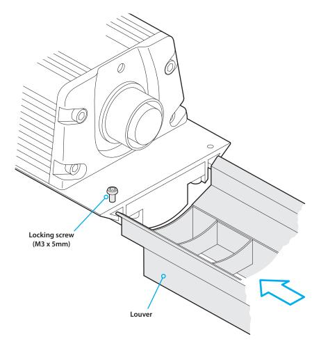
2 When the louver is fully in place, on the underside of the fixture, insert one of the supplied small locking screws at either end (on opposite sides) and tighten them to keep the louver firmly in place.
