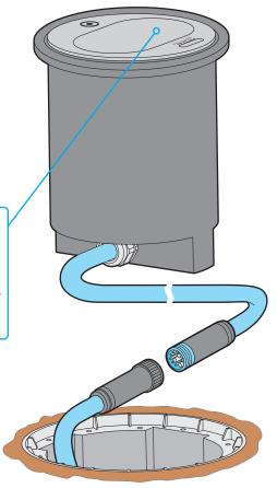
11 A small arrow (not fitted on direct ILLUMINATED frosted view models) is located under the top glass of the fixture to signify the tilt access. If the fixture will require fine tuning using the Terra-Tilt adjuster after installation, carefully Marker arrow rotate the fixture body within the chamber to ensure the arrow (or at least its axis) is pointing towards the object to be illuminated...
