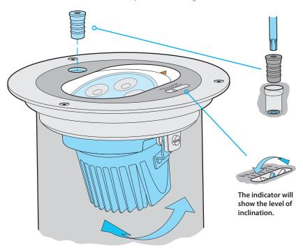
2 Use the Torx T20 driver to rotate the screw at the bottom of the aperture to cause the fixture head to rotate between +/- 15° until the surface is correctly illuminated.
