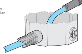
7 Prior to surfacing, replace the supplied pour cover onto the sleeve to prevent concrete entering the chamber. Tape over the hole in the pour cover.
