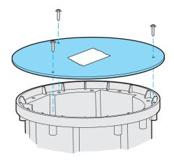
8 Once the finished surface has been applied, carefully remove the pour cover to reveal the chamber.
