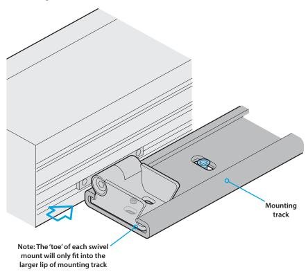
2 Slide the swivel brackets of the fixture into the mounting track and secure them at the required position using small grub screws.
