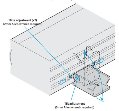
Ensure that each swivel mounting bracket is securely fixed to the mounting surface with appropriate screws/bolts. If necessary, use a 2mm Allen wrench to loosen the two grub screws on each swivel mounting bracket to allow them to slide along the length of the fixture to the required position before re-tightening.
