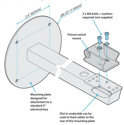
Note: When feeding cables through the extender bar, check for any irregularities that may have occurred during the manufacturing process - take care not to snag cables.
