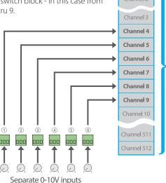
The complete DMX universe (including the six affected channels) is duplicated across all six of the DMX Out ports. Each port can drive up to 32 DMX devices.
