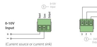
Port 1 of the 0-10V inputs is linked to the DMX channel chosen by the start address set by switches 1 thru 9 on the switch block. The remaining five 0-10V inputs are linked to the next five consecutive DMX channels.
