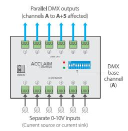
This diagram shows the inside story of the 0-10V to DMX conversion. The six separate 0-10V inputs are converted into equivalent digital values (each between 0 and 255). These are then applied to the six DMX channels that are selected by the switch block - in this case from 4 thru 9.
