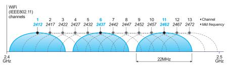
Aria uses the IEEE802.15.4 standard, with channels that are 3MHz in width and do not overlap. Many Aria channels do, however, coincide with the common WiFi channels. The notable exceptions are Aria channels 4, 9 and 14, which fall into the gaps between the most commonly used WiFi channels:
