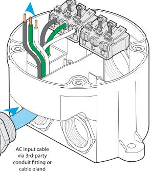
6 In turn, insert the incoming live, earth and neutral lines into the AC IN connector block, alongside and matching the connections from the internal surge protector.
