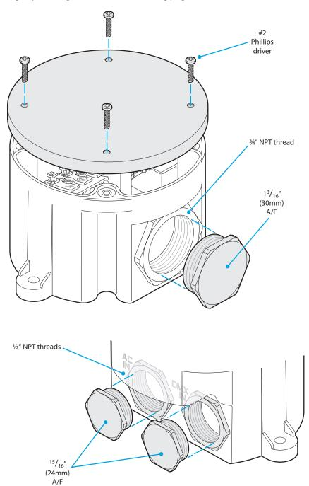
2 If required, gently prise off the rubber seals from the blanking plugs using a small flat blade screwdriver in order to install them on the cable glands/conduit fittings that you're using:
