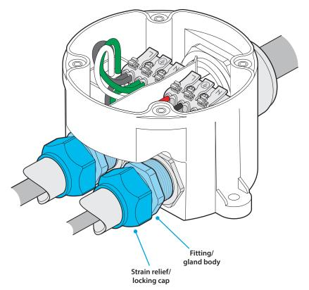
16 Push each cable slightly into the box (to ensure there's sufficient slack inside) and then tighten the strain relief/locking caps of the fittings/glands using an adjustable wrench.
