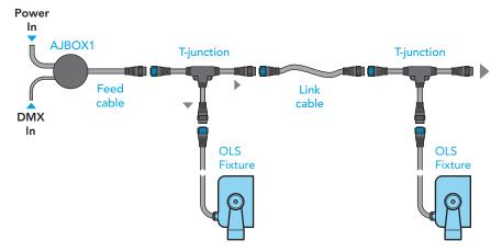
At the first T-junction, one output supplies power and control to the first fixture while the other continues to the next T-junction (either directly or via a link cable), where the process is repeated. At the end of the run, a terminator plug is fitted to simultaneously protect the live connections and correctly terminate the DMX control feed.
