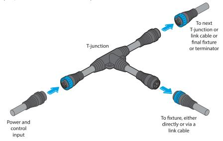
The blue collars form the locking and release mechanism:
