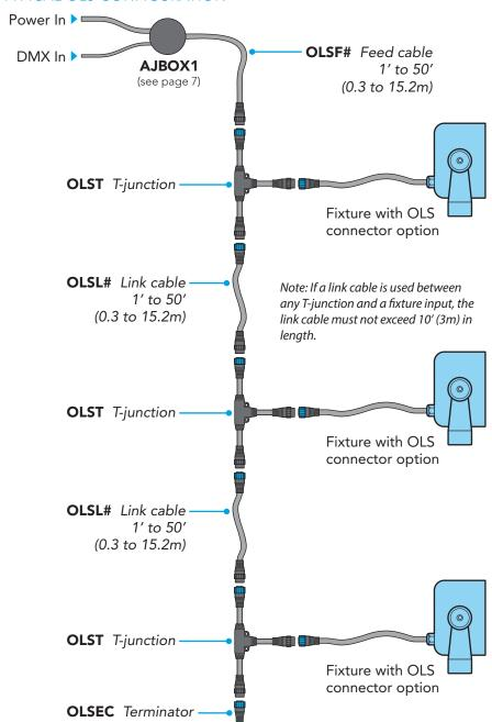
IMPORTANT: A terminator must be fitted to the final T-junction to simultaneously protect the live connections and correctly terminate the DMX control feed.
