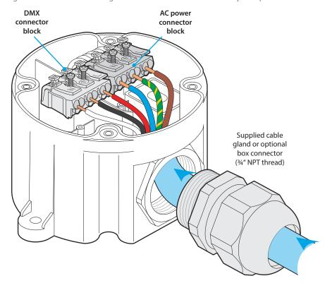
9 In turn, insert the six OLS feed wires into the AC power and DMX connector blocks, taking great care to ensure that the various wires are mated only with the correct terminals (see page 8 for wire designations):
