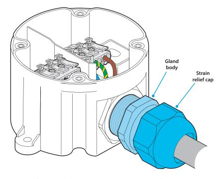
13 Push the OLS feed cable slightly into the box (to ensure there's sufficient slack inside) and then tighten the strain relief cap of the gland using an adjustable wrench.
