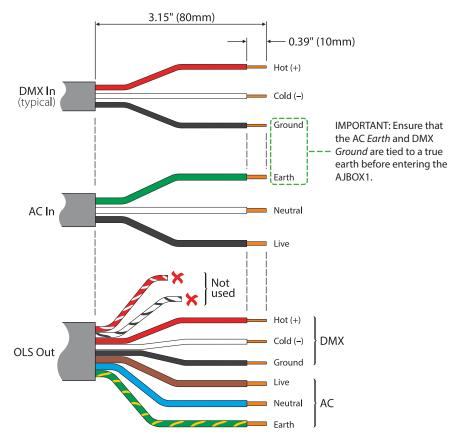
The DMX hot and cold out connections (red/white and white/black striped) are not used and can be trimmed. We suggest that you cut them short at slightly different lengths and ensure that no conductors are visible. Optionally you could also cap them off. Double check that they cannot short together and are well away from the mains connections.
