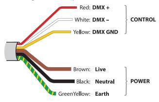
Control cores: 24 AWG / 0.25mm<sup>2</sup> Power cores: 14 AWG / 2.5mm<sup>2</sup> IMPORTANT: Ensure that power earth and DMX GND are both tied to true earth.
