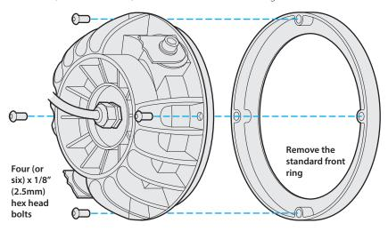
2 Replace the front ring with the trim ring supplied with the optional In-grade housing kit. Use the four (six) bolts removed earlier to secure it:
