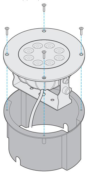
6 Insert the four supplied screws and use a TA2.3mm triangular driver to tighten them.
