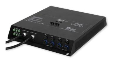
XTR Driver 8000™ is a specialized module that powers continuous runs (up to 700′/213m) of high intensity linear LED fixtures. XTR Driver 8000 features dual 220V-277VAC power inputs, a clear display for control input selection and up to 8000W of high voltage DC output power. The following control formats are all supported: DMX-512A, DALI or 0-10V/1-10V. All connected linear LED fixtures must conform to the Acclaim Lighting XTR Link standard.
